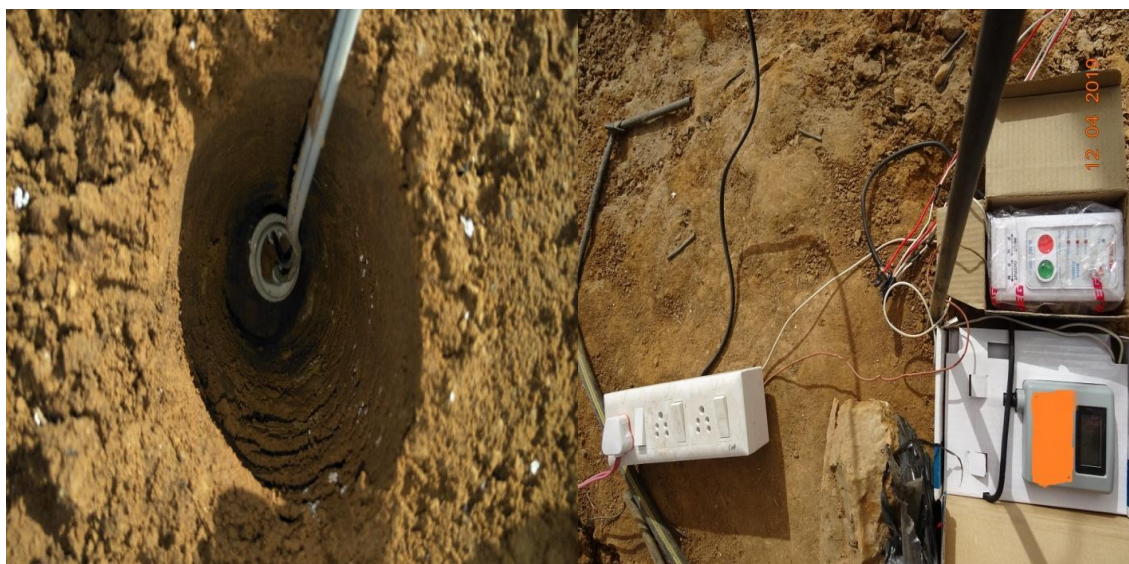
Fig. 5: Experimental view of sensor and automated drip system.
